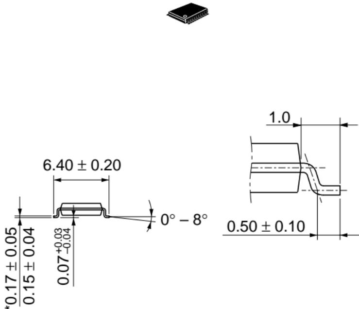
\*Dimension including the plating thickness
