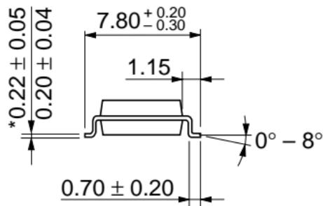
\*Dimension including the plating thickness
